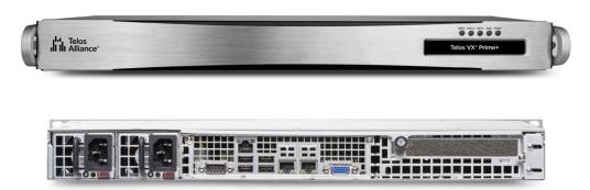
The heart of any VX system is the Engine. The fixed-capacity VX Prime+ system is powered by a 1RU rack-mount Engine with enormous processing power. In fact, the VX Prime+ Engine provides all the call control and audio processing needed for your entire on-air phone system.
